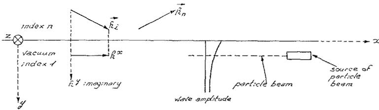
Fig. 6. Beam of particles undergoing transitions inside Fresnel's evanescent wave.
