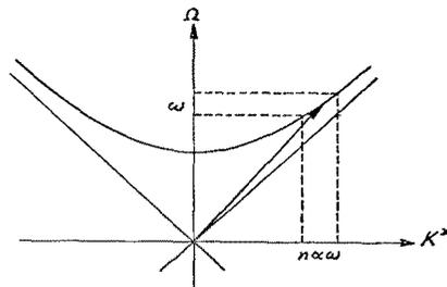
Fig. 7. First-order photoelectric effect on free electrons.
