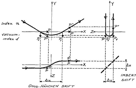
Fig. 5. Total reflection of a spinning photon (positive helicity).
